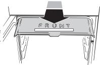
The side panels of the main oven can be removed.
